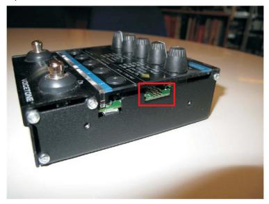
Use Midi OX to upload the hex. file which you can find on the technical server. The footswitch LED's starts flashing while receiving the data. After the data has been send the product will boot up by itself.
