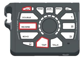
2 Turn the encoder, and press the lit buttons to step through the front test which tests all buttons/LEDs.
