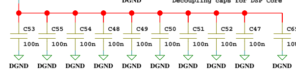
Decoupling caps for DSP Core
