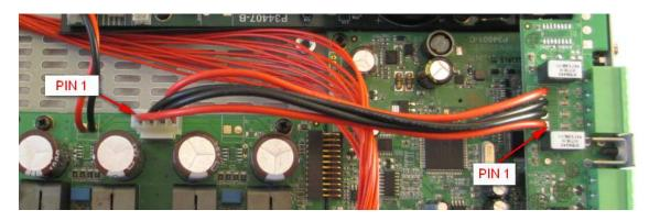
The correct mounting of the wires. Pin 1 to pin 1. 2 to 2, 3 to 3 and 4 to 4. That can be done either by unsoldering the wires for relocation or to unplug and replace in the connector.
