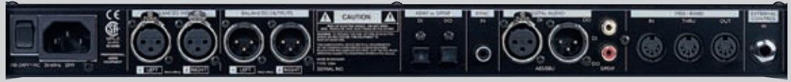
Main Power Switch Power Input 100 - 240V Balanced XLR Analog Inputs Balanced XLR Analog Outputs Digital In/Out ADAT Tos-link Word-clock RCA Digital In/Out AES/EBU S/PDIF MIDI In,Thru,Out External Control Input
