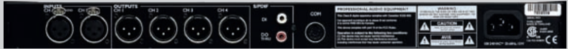
Balanced Inputs on XLR for channels A/B. Use channel A for mono Input. Balanced Outputs 1-4 on XLR. Digital S/PDIF In and Thru on RCA phono. Com port for data transfer. NO user application. Power Input. The internal switchmode powersupply accepts from 100 to 240 VAC.
