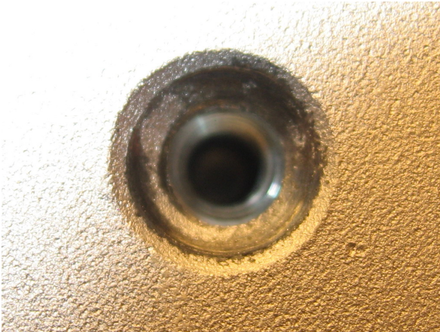
Figure 44: Align all the 3mm press nuts with the holes in the “Top Cover” as shown in the picture.
