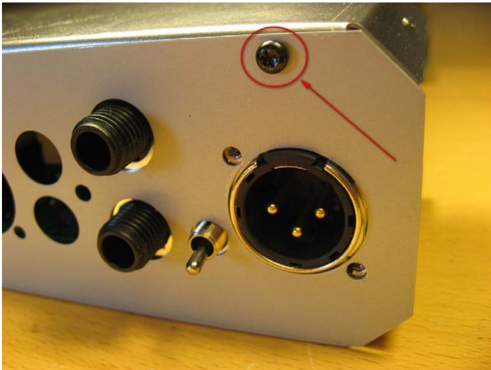
Figure 32: Mount one M2.5x4.5 torx8 as shown in the picture.
