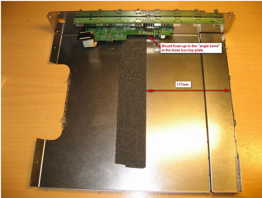
Figure 29: Mount the foam in the “inner box top” parallel to the side.
