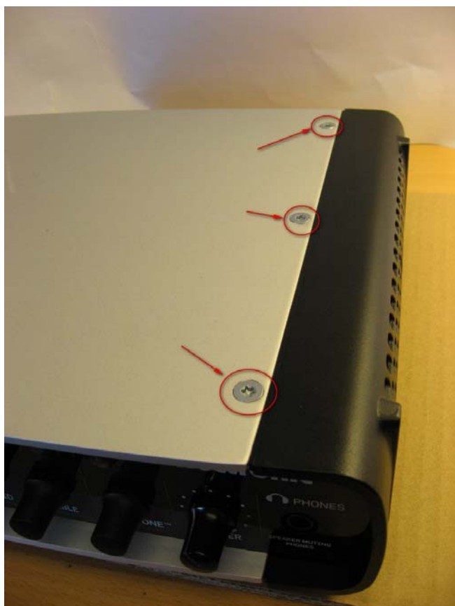
Figure 49: Mount the three screws as shown in the picture. (3 pcs. M5x7 torx black)
