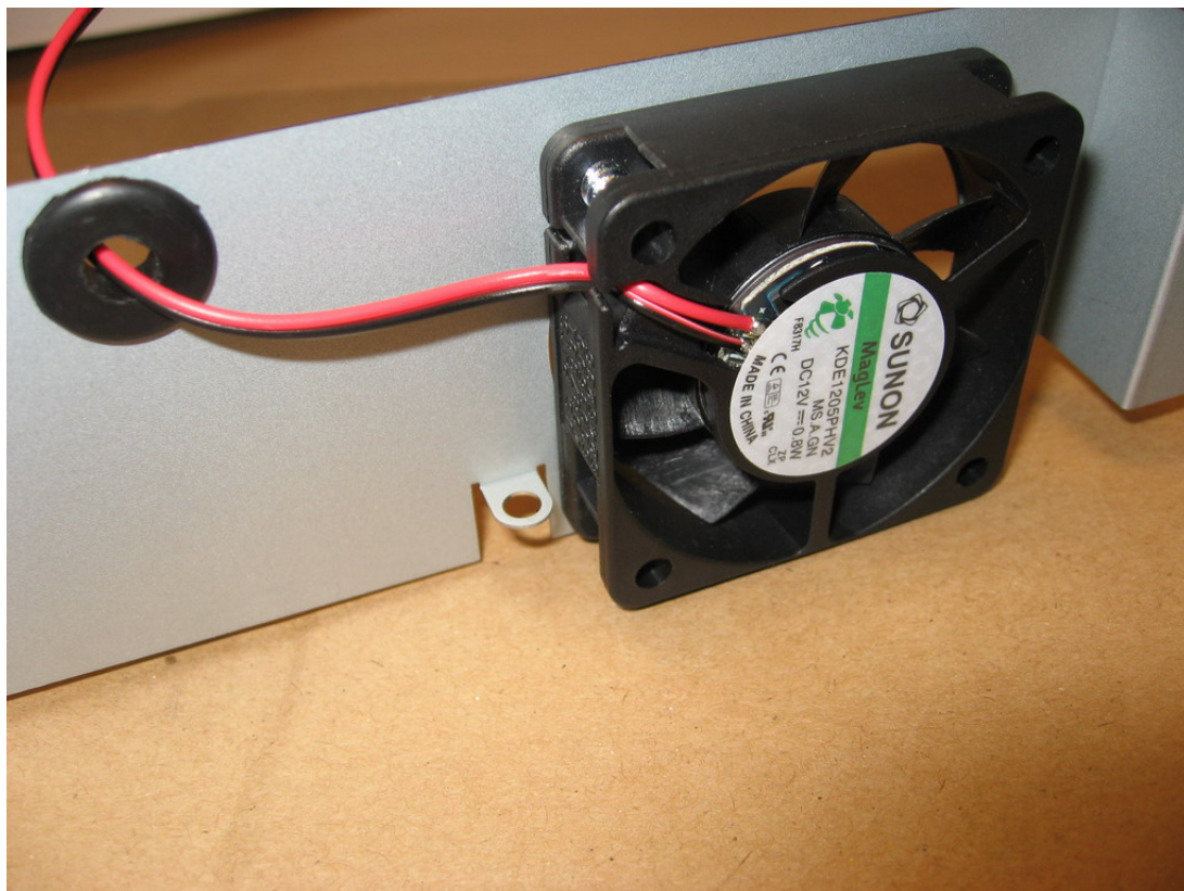
Figure 5: Mount Rubber-Grommet and Fan as shown in the picture. It is important that the fan is positioned correctly due to the direction of the air flow.
