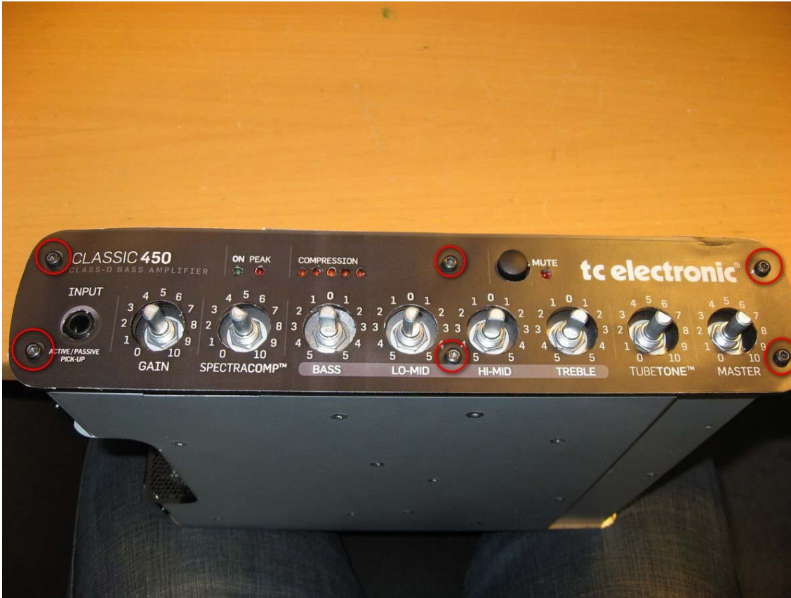
Figure 40: Mount front plate using 6 pcs. M3x6mm screws as shown in the picture.
