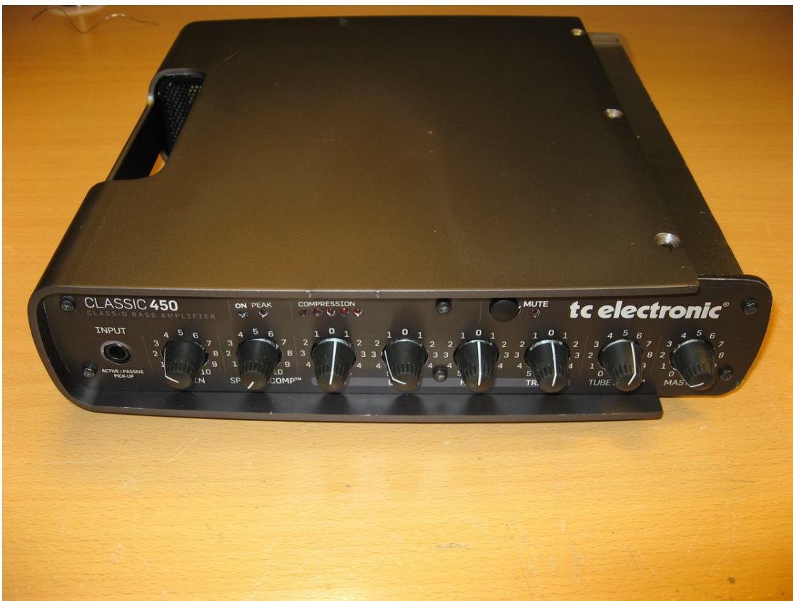
Figure 43: Make sure the frontplate fits into the groove all the way round the top cover as shown in the picture.
