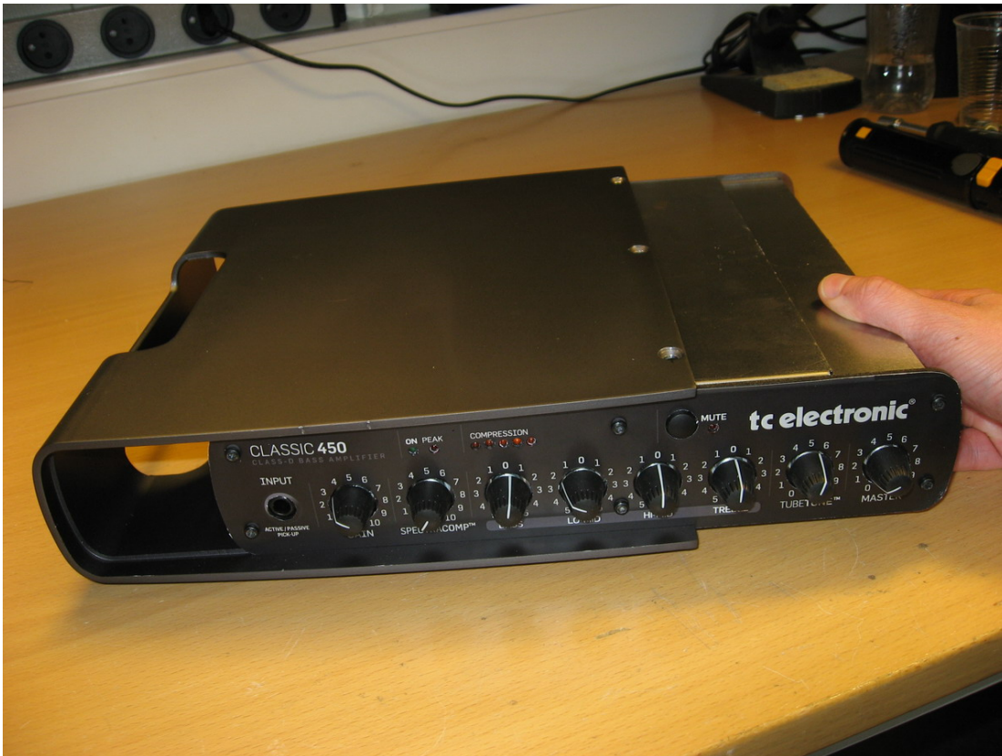
Figure 42: Slide inner box into top cover as shown in the picture.
