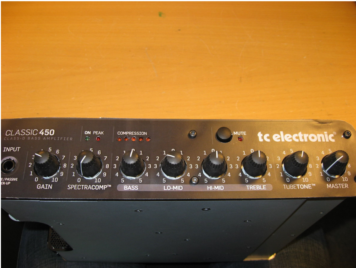
Figure 41: Mount 8 pcs. "DR09803, plastic knob for pots 112 Dirch" as shown in the picture.
