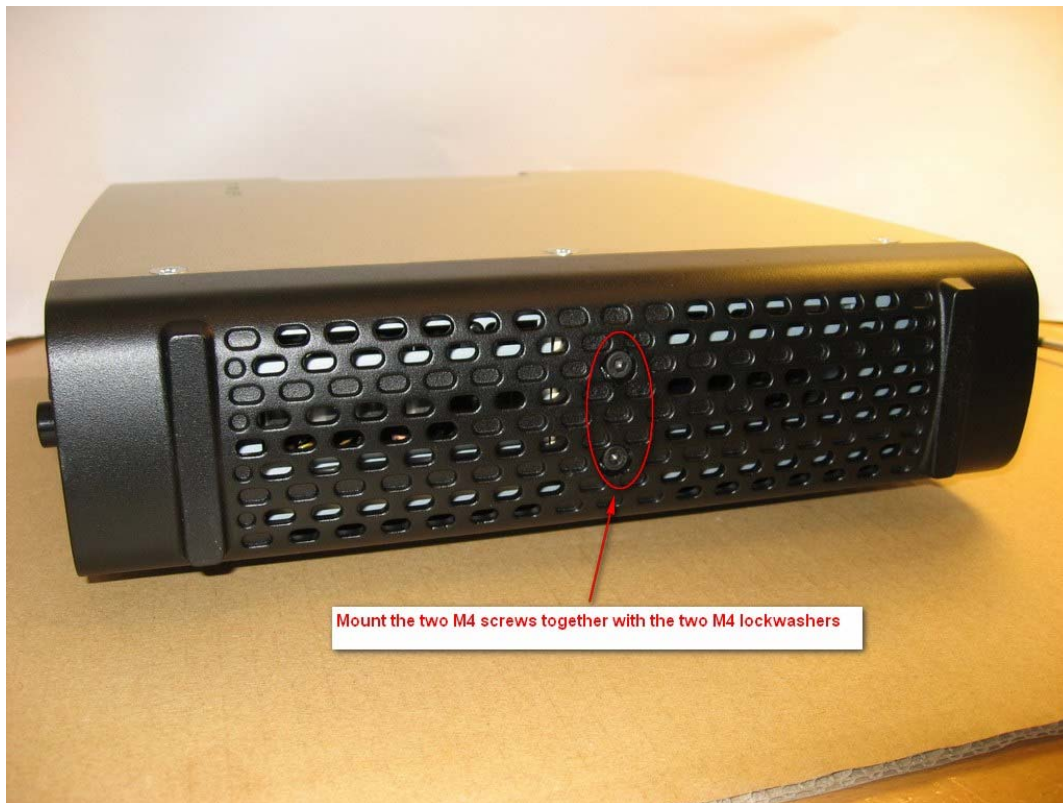
Figure 50: Mount the two screws and two lock washers as shown in the picture.
