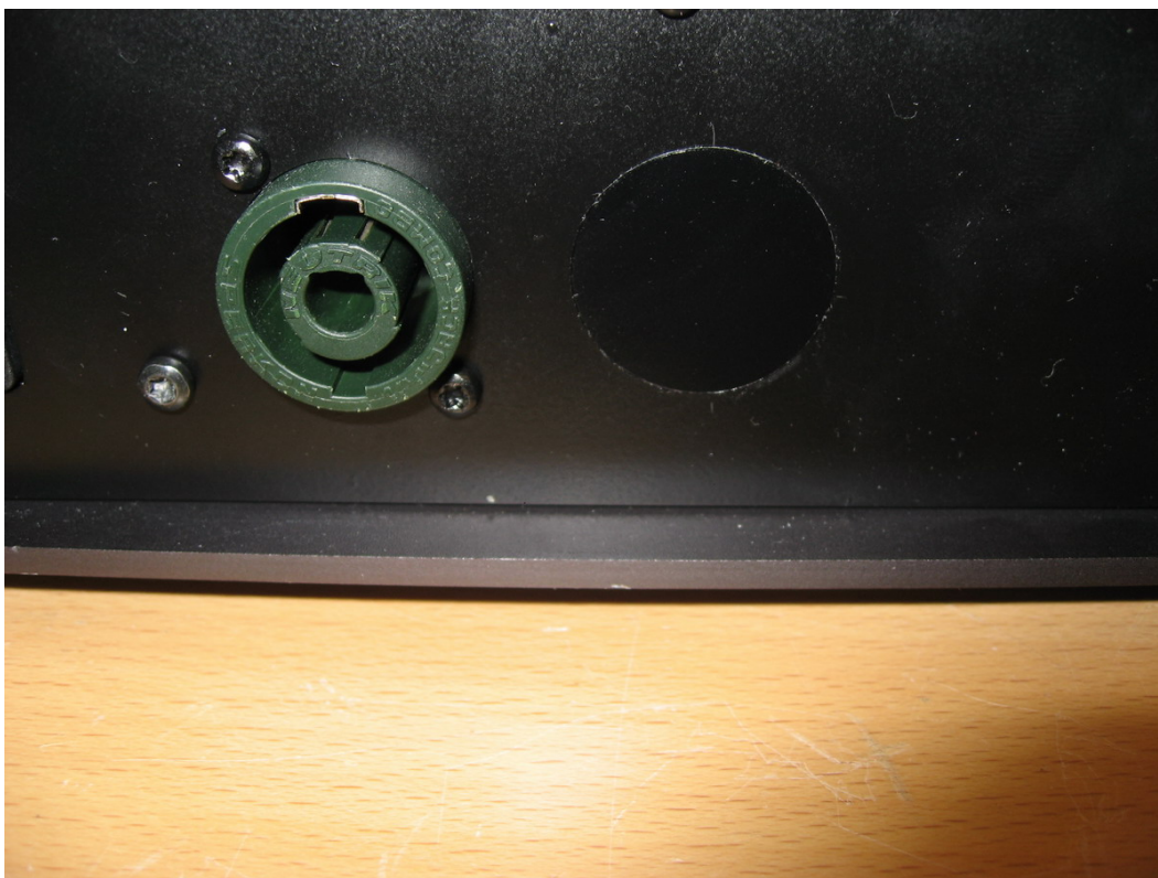
Figure 51: After final test mount the E58209011 “DR09027-A, Sticker for MIDI-port, 1112 Dirch“ to cover the midi port. As shown in the picture.
