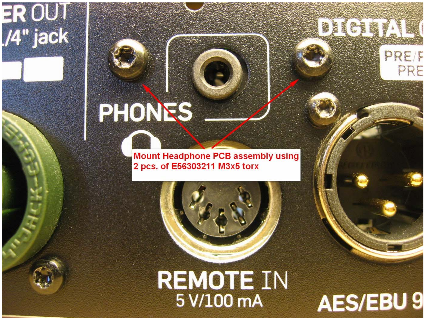
Figure 4: Mount the P18507 headphone PCB using two screws as shown in the picture.
