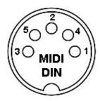
Pin 1 +5V Pin 2 GND Pin 3 shorted to pin 5
