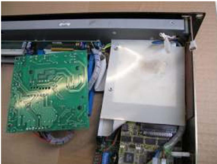
Remove the Floppy disc drive and all the cables for this.
