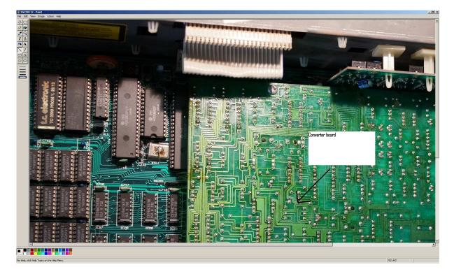
No effects: Can be the converter board that's defective; use your test converter board to check it.
