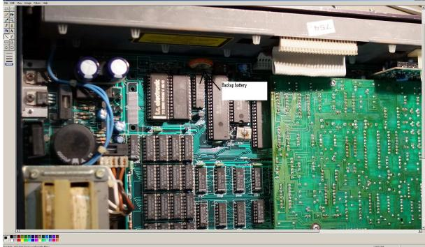
Always hard wire the power supply wires from the transformer going to the main pcb.
