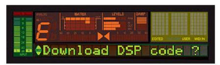
✓ Press **MENU**to confirm. The display now reads "Downloading code 000" which means the Triple C is ready to receive the update.
