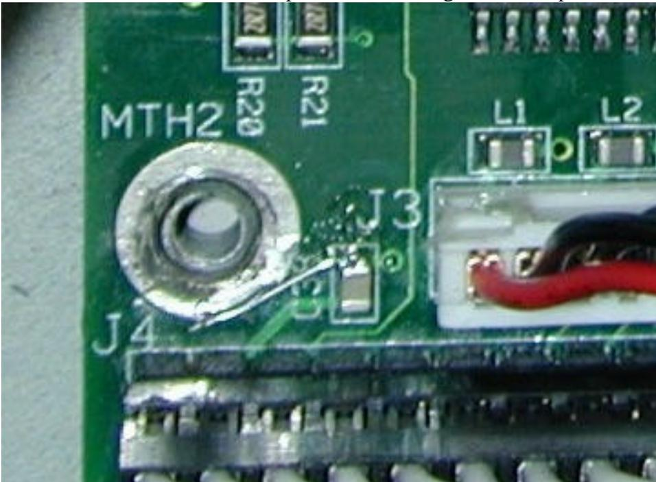
5. Replace the screw back to position MTH2 and put cover back on the VoicePrism Plus.
