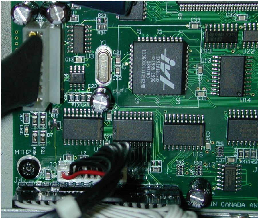
3. Remove machine screw from MTH2 as shown below
