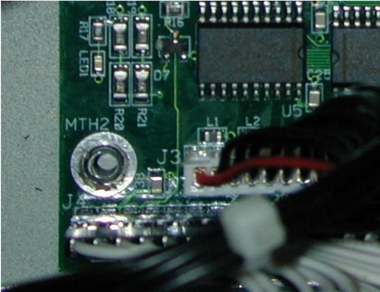
4. Solder a wire from the top of C38 to the edge of MTH2 pad as shown below
