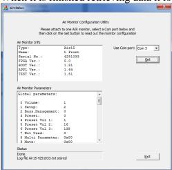
In the top window it is possible to see type, task serial number and software versions. If one or more of the software versions are lower than the latest release, it is highly recommended to do an update.
