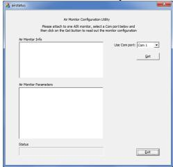
The program it self is quite easy to use, simply set the Com port used on the PC and press the "get" button. –Remember that the monitor must NOT be connected in a network!
