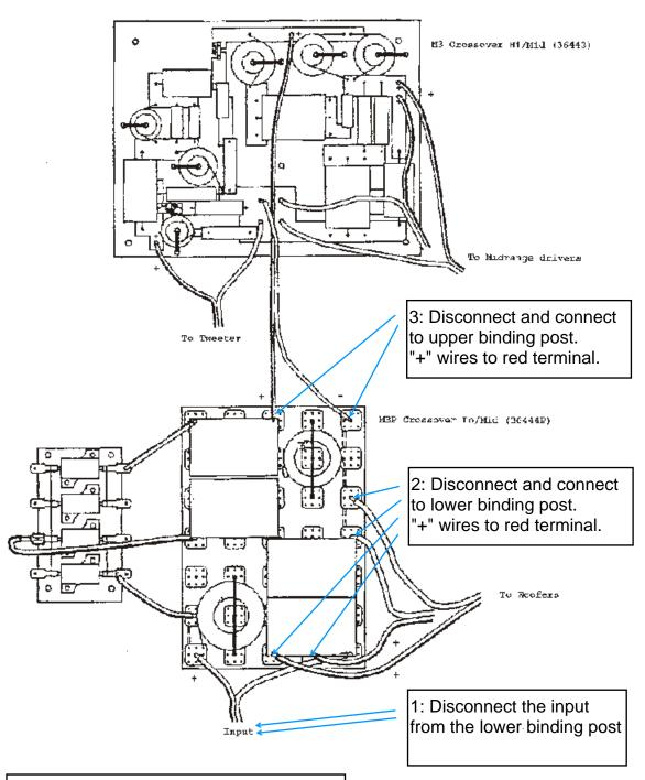
4. Mark the upper binding post: "Mid/Hi" and the lower binding post: "Low"
