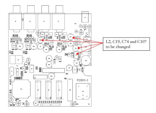
Our tests show that the Nova pedals by this change can handle incoming supplys from 8.5V.
