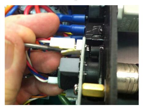
■ Set the wires straight and place a snap-on ferrite over the cable:
