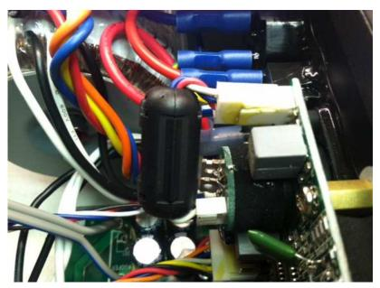
■ Place a second snap-on ferrite on the cable interconnecting the pre-amp board to the output/PSU board:
