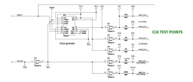
If RESET Line is being constantly asserted (Active-Low), it could be an issue with the filter capacitors in the 3V3+ Line. Using an oscilloscope, check CLK points for DSP1, DSP 2, AVR and DICE. If you notice patterns such as;
