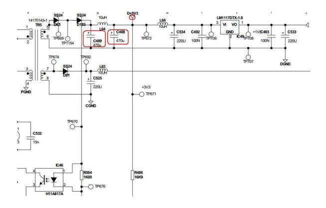
Locate these 2 capacitors (they're to the right of the SMPS solder points) and place your oscilloscope probe on the top of each one. If a similar oscilloscope readout to the previous RESET line status, then try replacing these 2 caps. Go for at least a 10V/105 Degrees value electrolytic.
