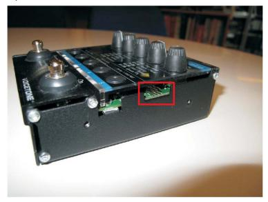
Use Midi OX to upload the hex. File which you can find on the technical server. The input led will light up red while receiving the data. After the data has been send the product will boot up by itself.
