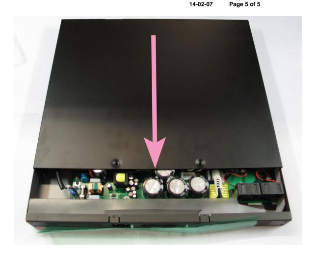
Inspect that fan havent tilt by looking in with a flash light trough the front grill
