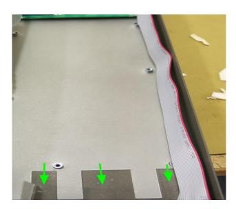
4. Remove one of the protective sheet and mount them according to the picture below. Then remove the protective sheets from the top off the foam sticker.
