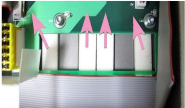
Place the fans on the adhesive foam stickers and press down (pink arrows). Make sure that the stickers of the fans are placed in the direction that the white arrows show. Also check that the fan-cables come out from the sides according to the green arrows. Mount the connectors on the mounting headers according to orange arrows. Make sure that fan-cables are not stuck in the fans.
