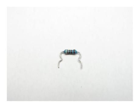
Mount the new resistor as shown in the picture and make sure the resistor don't make contact with any component's or PCB.
