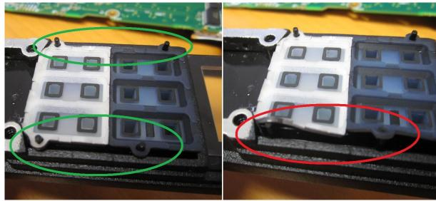
3. Put back the front panel PCB and confirm that all nibs are ok.
