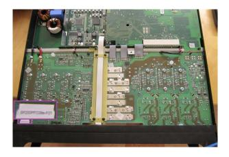
6. Remove screw from the bottom cover. Remove the cover.
