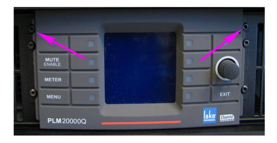
13. Remove the front panel from the chassis.
