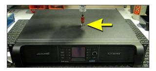
5. Remove the screws holding the DICO support.
