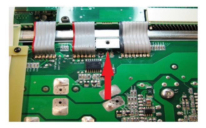
9. Check for scratches on the lead, if it is broken try to repair the lead before you continue to the next step
