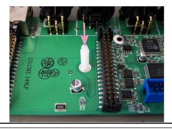
4 Mount the DSP-board back on to the ADIC board
