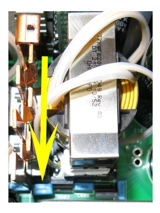
7. This is the faulty capacitor it's the grey vishay capacitor. If you find this capacitor follow the instructions below on how to replace them
