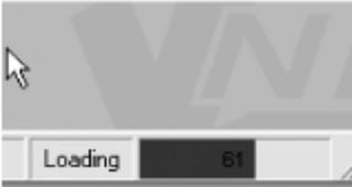
9. After the download is complete the following message appears. The DSP is updating at this point. Do not power down the unit or disconnect any network cable at this point. During the update a red bar will show the progress of the firmware update (bottom right of screen).
