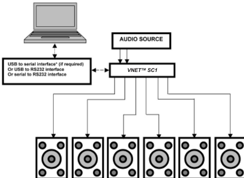
\* USB to Serial interface allows networking of multiple VNET™ speakers or SC1 controllers
