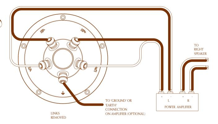
Please note in bi-wire mode that the link plates should first be removed.
