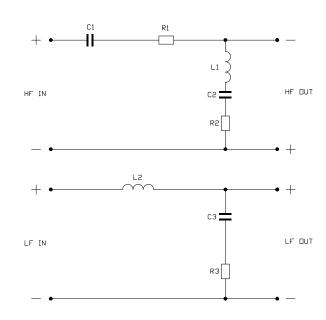
\* L1 CAN BE MADE SMALL, BUT ADJUST VALUE OF R2 TO COMPENSATE FOR DCR
