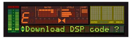
✓ Press **Enter** to confirm. The display now reads "Downloading code 000" which means the D-two is ready to receive the update.
