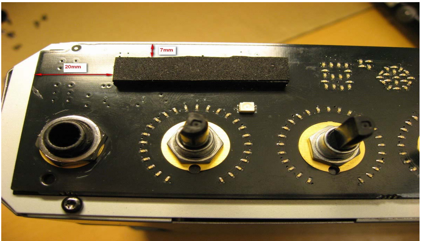
Figure 52: Mount one pcs. of “DR09022-A, Foam for Window” as shown in the picture.
