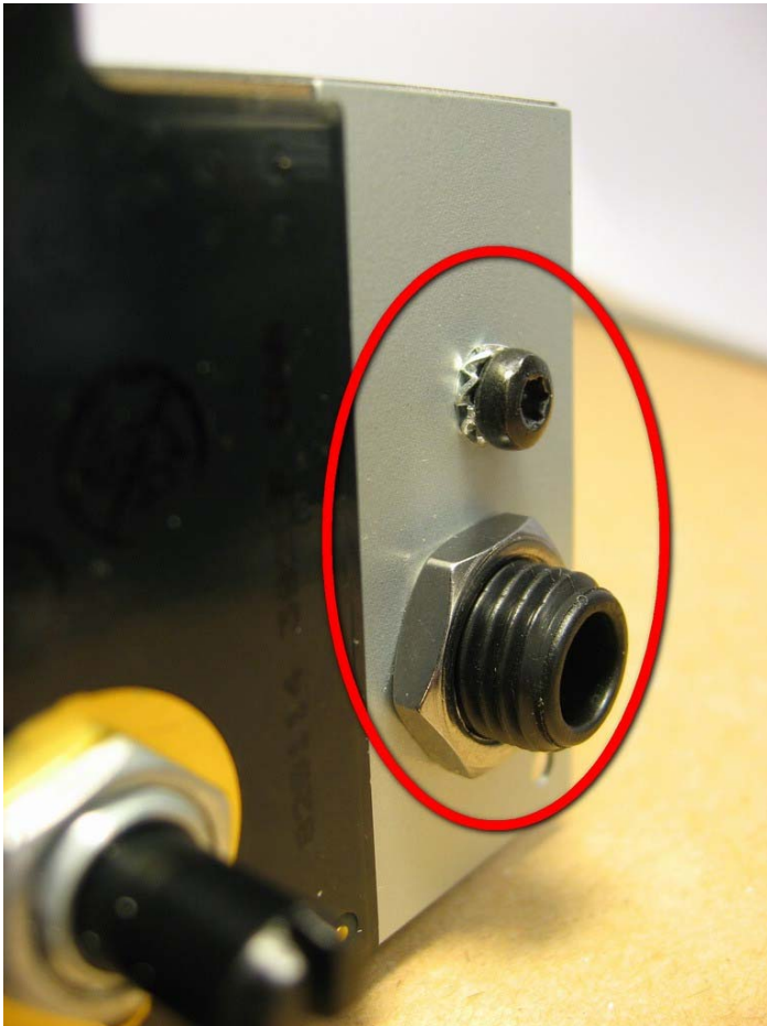
Figure 31: Mount the Headphone breakout PCB using the M3x5 screw, the 3mm star washer and the hex nut as shown in the picture. The hex nut must be tightened using 7,5 kgf*cm (0.7 Nm) force. Thread lock must be used on hex nut!
