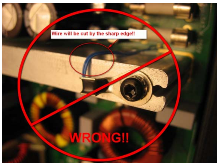
Figure 13: Be sure to mount the sensor correctly!! This is WRONG.
