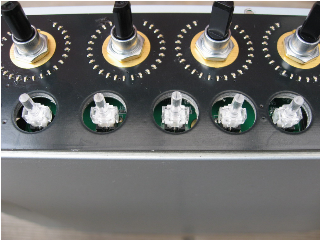
Figure 26: Mount 5 DR09012, Switch Lightpipes as shown in the picture.
