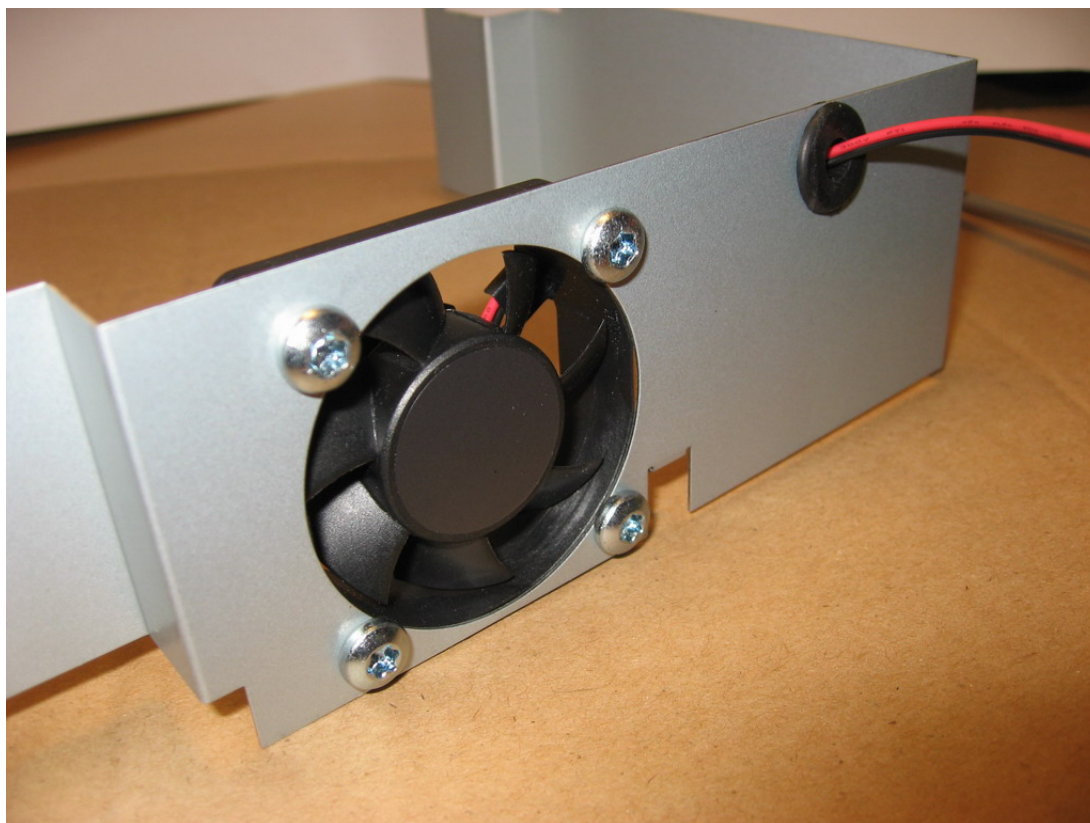
Figure 6: The fan is mounted using the 4 screws M4.8x13 E56306211.
