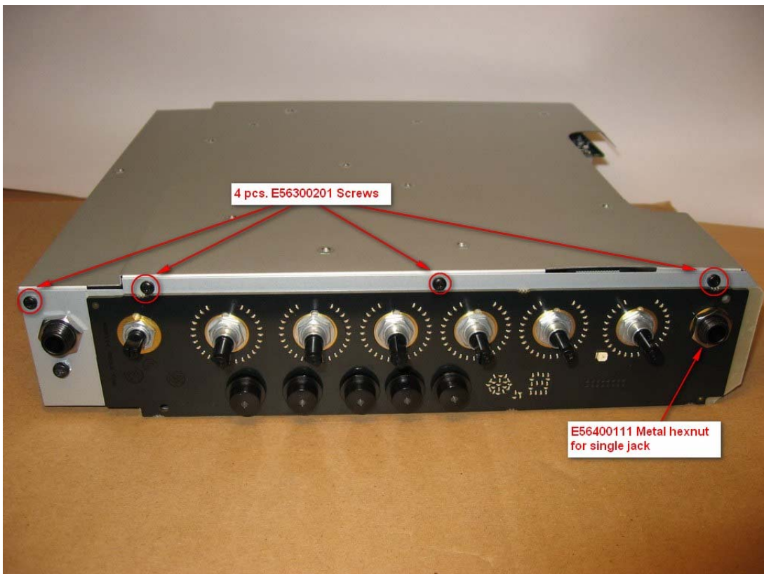
Figure 42: Mount four screws and one hexnut at the front side of the product as shown in the picture.
