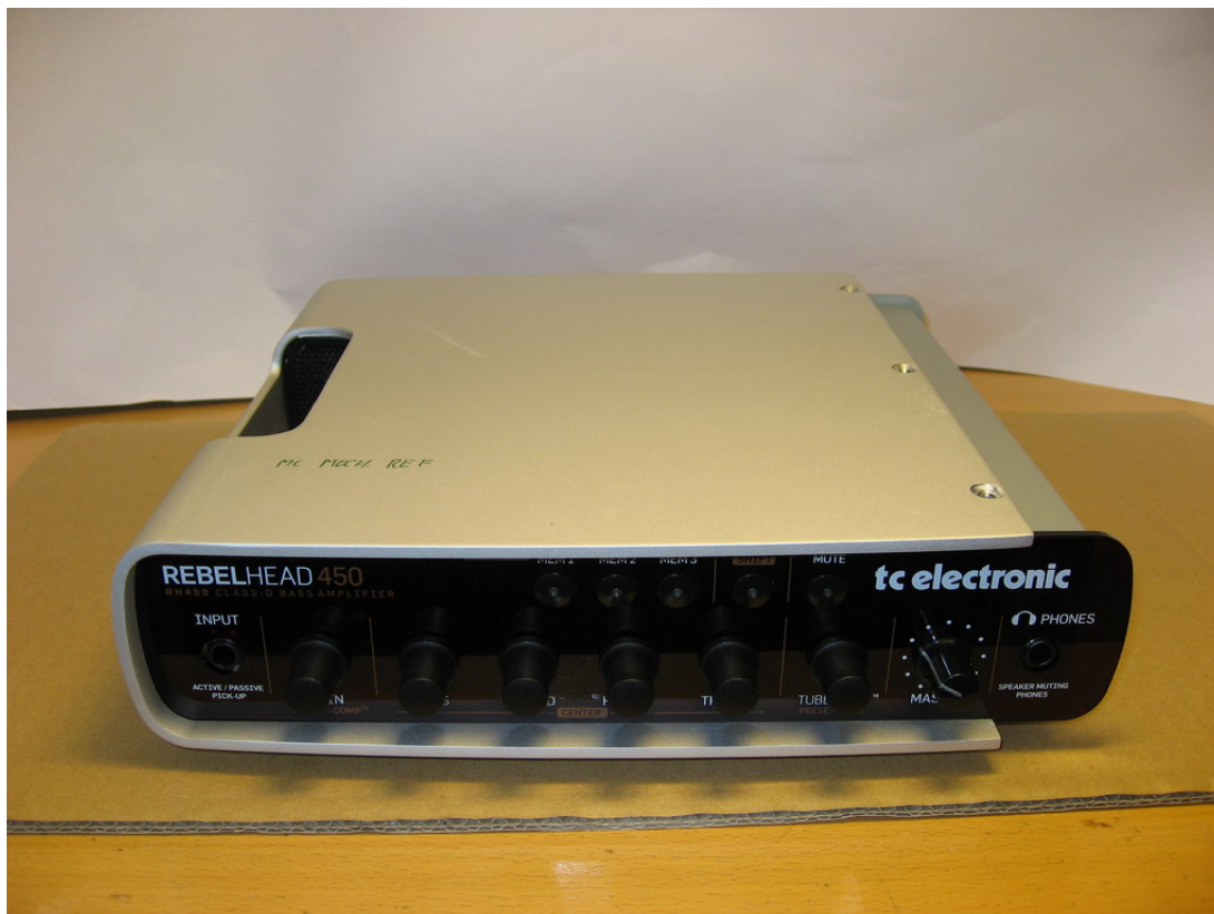
Figure 57: Make sure the window fits into the groove all the way round the top cover as shown in the picture.
