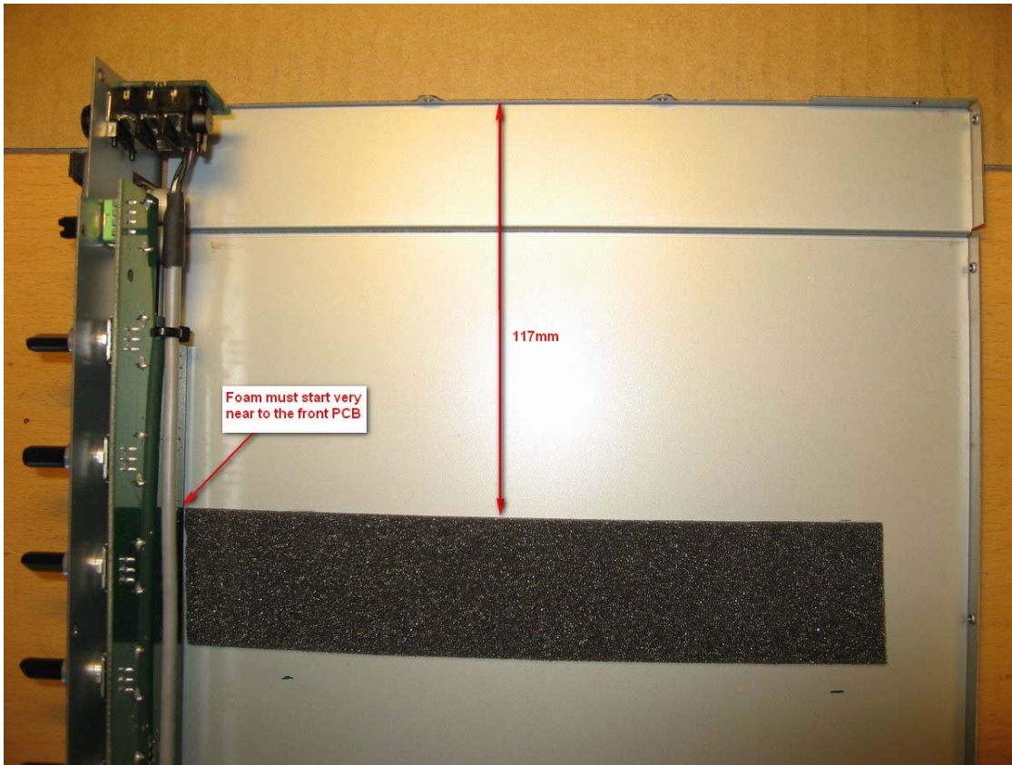
Figure 37: Mount the foam in the “inner box top” parallel to the side.
