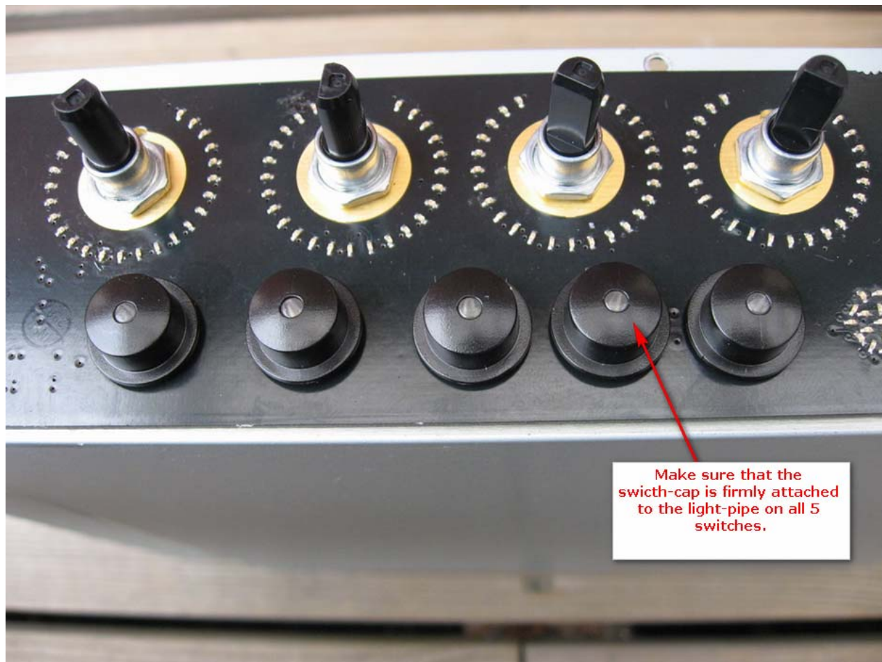
Figure 28: Mount 5 psc. of DR09011 Switchcap as shown in the picture.
