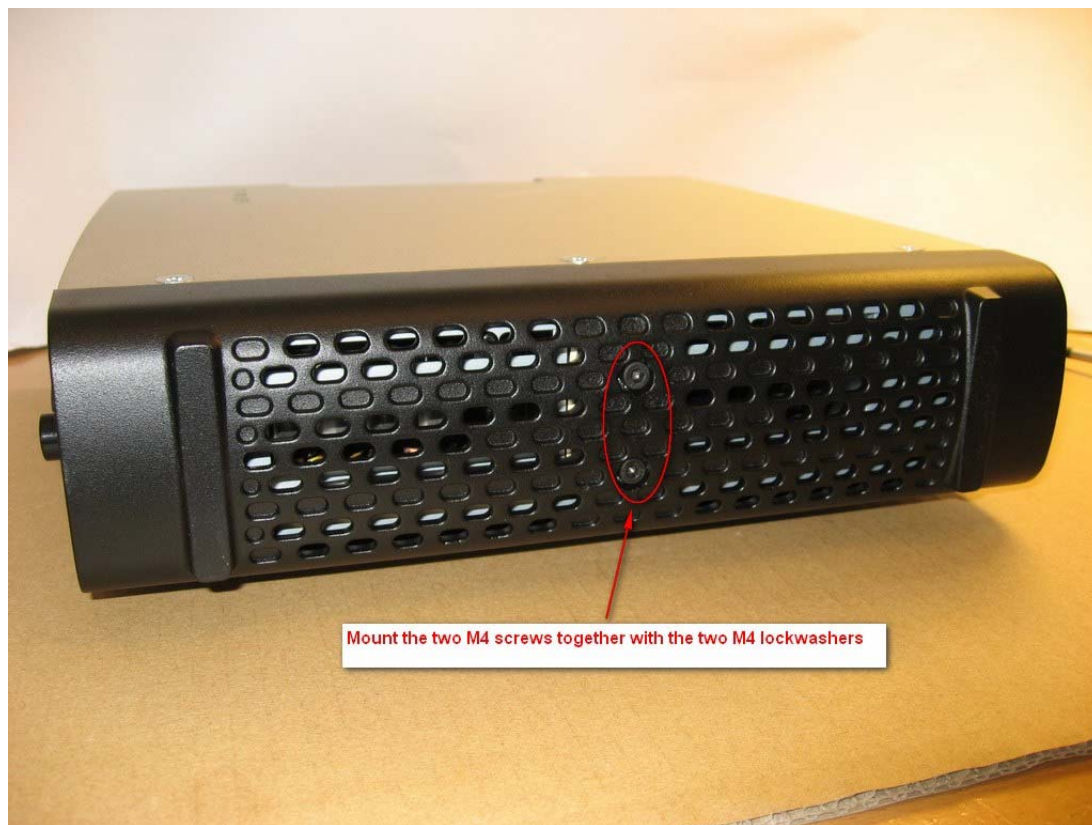
Figure 64: Mount the two screws and two lock washers as shown in the picture.
