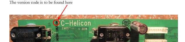
The footswitch PCBA board (with footswitches mounted) can be ordered from TC. Please remember you need 2 boards for one VoiceLive 3.
