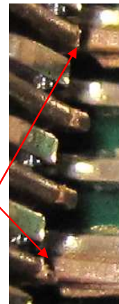
Holdes for the bottom plate are broken off.
