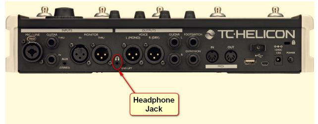
1. Locate the headphone jack on the back of the VoiceLive 3 device.
