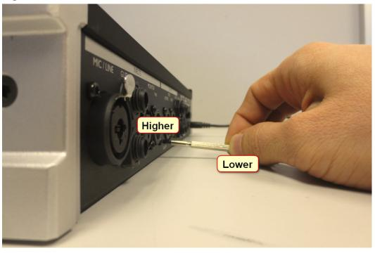
Once the switch has been located, push it in while powering up the VoiceLive 3. If you see the below screen then you have successfully reached the maintenance mode.
