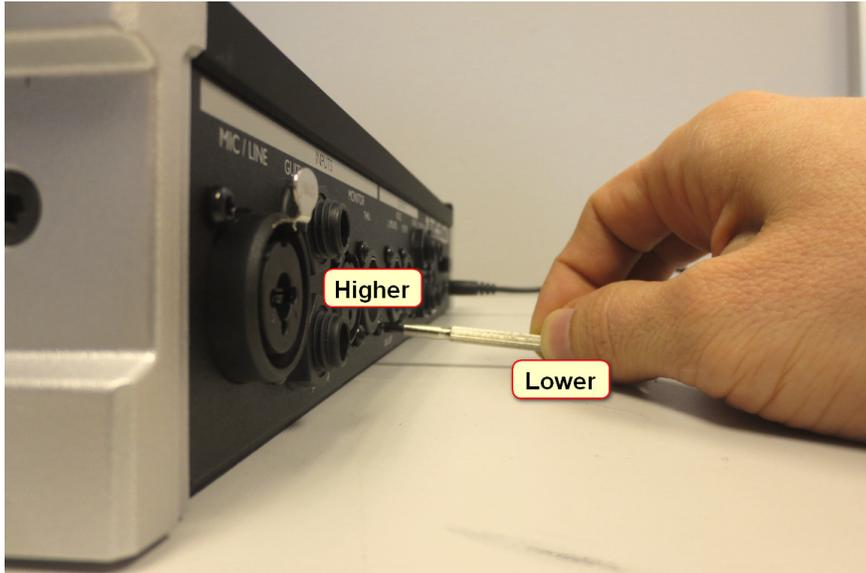
6. Once the switch has been located, push it in while powering up the VoiceLive 3 (make sure USB stick is inserted). If you see the below screen then you have successfully reached the maintenance mode.
