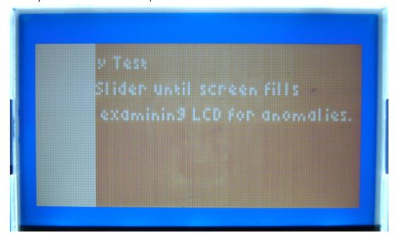
7. The front test is now complete and the following screen will be displayed. Power cycle the unit.
