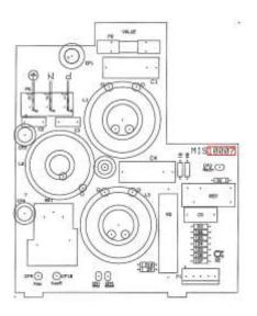
Picture below shows the placement for R19 on SP100F, SP130F and SP140F. The resistor on the SP130 and SP140 may already been disabled by a trace on the back of the board, make sure to check this before you disable any of the two resistors.
