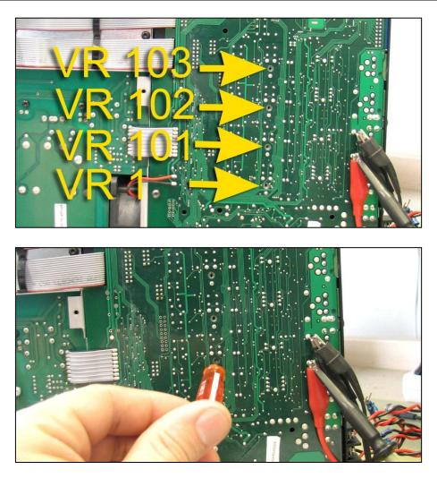
Connect speaker to Ch B. Adjust VR101 at AICO to minimum 100Hz. Listen to speaker.
