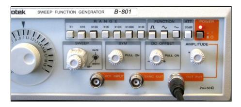
4. Check signal level at oscilloscope. Adjust signal from generator to ca 0,5V peak (0,35V Rms)
