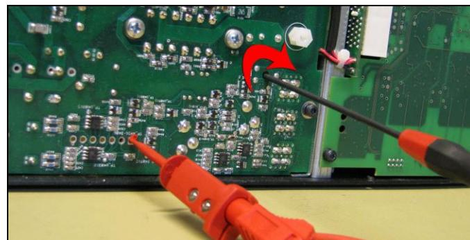
7. Attach multimeter for RAIL and use SG for reference (**Pic 1**).
