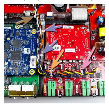
Remove the cables shown in the picture below
