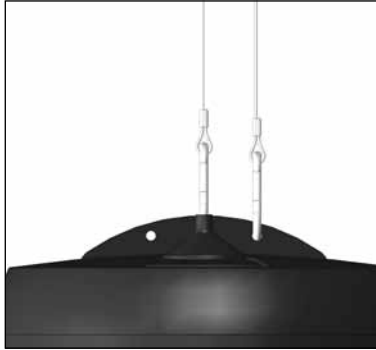
HANGING / SAFETY WIRES
