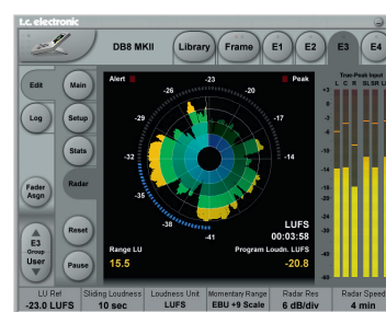
LM6 Loudness Radar Meter The DB4/DB8 MKII feature the new EBU R128 and ATSC A/85 compliant LM6 Loudness Meter
