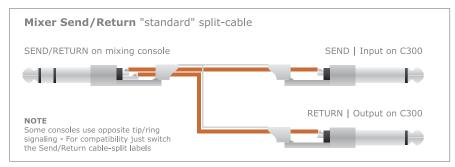
Type 1 and Type 2 cables are used when C300 is used as channel insert effects with mixing consoles that has unbalanced insert points on 1/4" stereo jacks.
