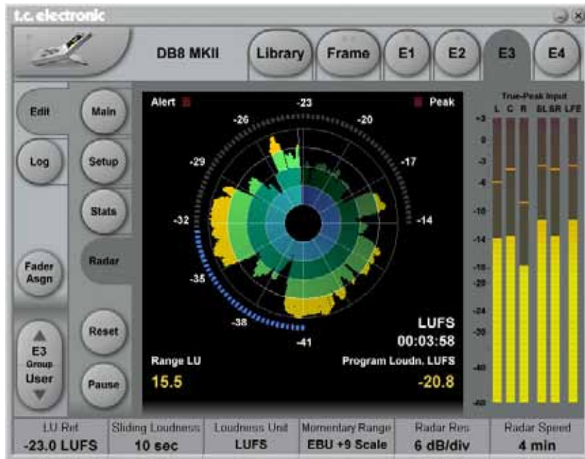
Fig 3 - Radar page features of LM6 in DB4 and DB8. Target Loudness is displayed at 12 o'clock of the outer ring, and at the bold circle of the radar indicated also by the transition from green to yellow. The descriptors Loudness Range and Program Loudness, are the yellow numbers in the lower part of the display. Press the Reset key to reset Radar and Descriptors.
