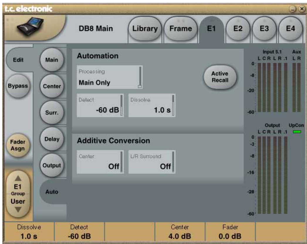
Fig 3. The Auto page parameters. Note green UpCon indicator to show up-conversion currently active.
