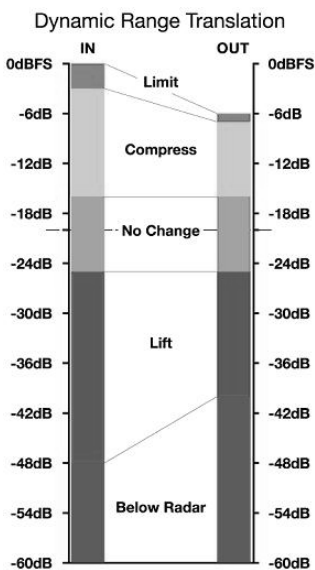
Fig 3. Example of dynamic range re-mapping: From Home Theatre/DVD to Living Room listening conditions (Fig 1). Fig 3 and Fig 4 show rational transfer characteristics complying with the DRT of the consumer, without affecting levels when they are already on target.
