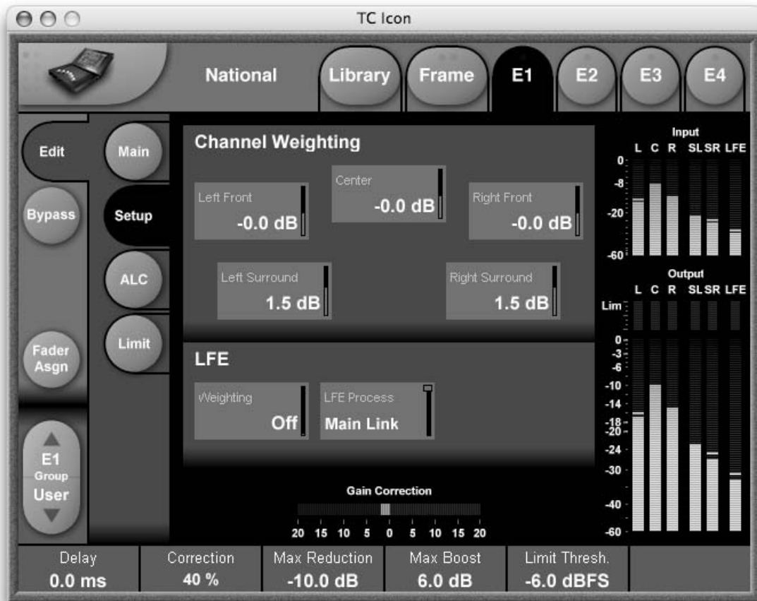
Fig 4 The Setup page of ALC5.1 showing settings according to ITU-R BS.1770.
