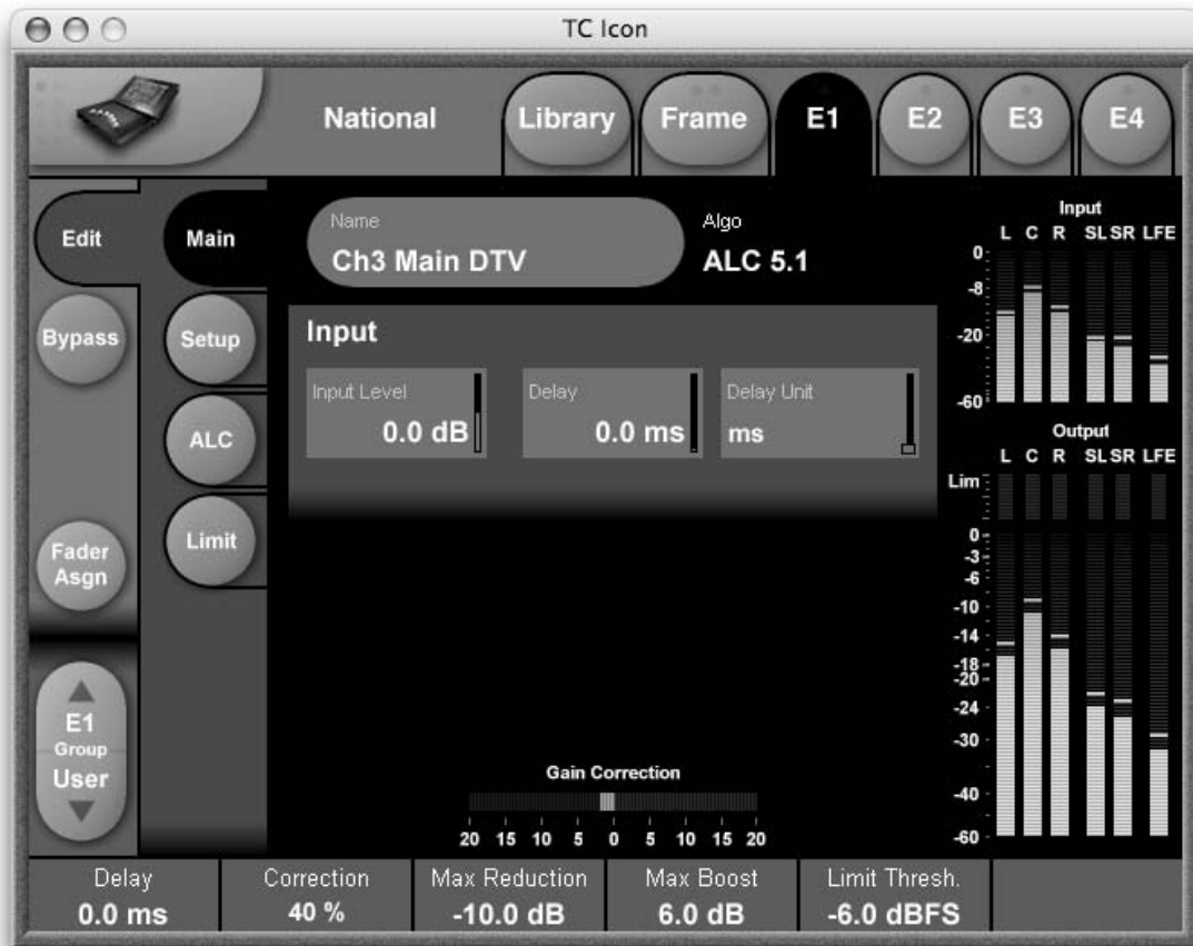
Fig 3 TC Icon view of ALC5.1 Main page parameters. Be sure to use Icon version 3.82 or higher when controlling ALC5.1
