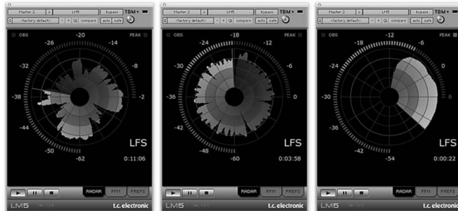
Fig 4 - Different types of program shown on the Radar Please note that these pictures derive from ProTools but measurements and radar display are identical to the ones found in DB4/Db8 and System 6000.
