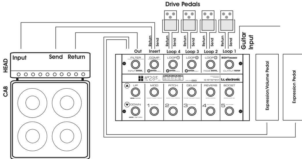
In this setup we are using a head as both pre-amp and power amp. The pre-amp section of the head is connected to the G-System's Insert loop. Set the Insert loop to "on" on all G-System presets, using the Utility menu.
