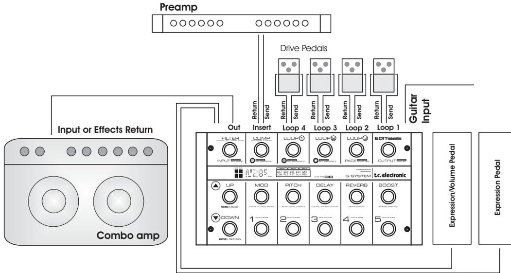
This setup is similar to the one described in the first example, but we have now added a pre-amp to the Insert loop. You can decide to have the pre-amp in or out of the signal chain per preset, but you will probably prefer to have it “on” at all times. This is configured in the Utility menu, which you can access in Menu Mode.
