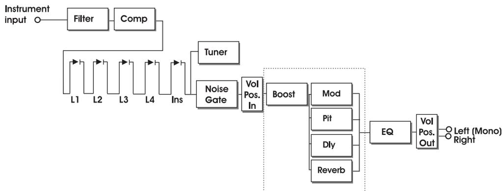
In the Parallel routing, the same signal is fed to the input of the Modulation, Pitch, Delay and Reverb sections, and therefore these effects will not affect each other.
