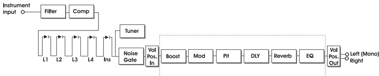
The Serial routing connects all Effect Blocks “in a straight line”, similar to a regular guitar stomp box setup. This means that each Effect Blocks affects the following effect(s).
