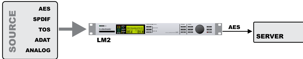
Fig 5 Meter and gain normalize for broadcast Ingest and QC. Use a preset from the Ingest bank.
