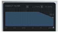
There are two frequency values indicated above the display: The "S" value is the start frequency of the high cut filter, which is the lowest frequency influenced by the filter. The "E" value is the end value. This frequency is where vou have reached the determined attenuation.
