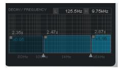
For each band you can set the decay time between 0.25 and 64 seconds. Use the Shift key to ungroup the decay times.
