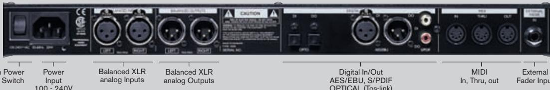
Main Power Switch      Power Input 100 - 240V      Balanced XLR analog Inputs      Balanced XLR analog Outputs      Digital In/Out AES/EBU, S/PDIF OPTICAL (Tos-link)      MIDI In, Thru, out      External Fader Input
