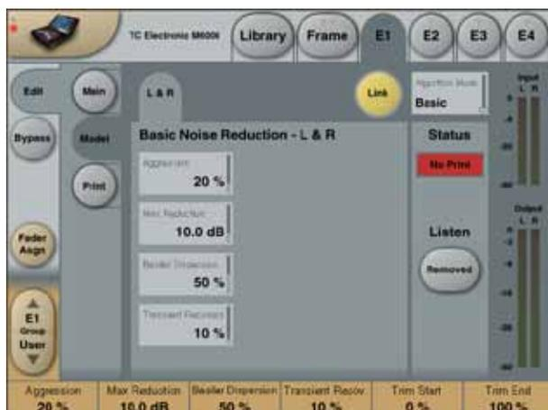
The Basic model offers the simplest set of controls for BackDrop. With the Basic model the noise reduction is applied to all components of the noise and across the entire frequency range. The Basic model is a good choice when the level of the noise is relatively low and when it is not very complex, such as tape hiss. The Basic model provides four controls (Aggression, Max Reduction, Basilar Dispersion, and Transient Recovery).
