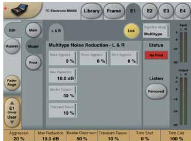
The MultiType model offers a unique and exciting new approach to noise reduction. The MultiType algorithm is based on the realization that most noises are actually a sum of several different individual noise components. Moreover, the noise components may not be equally annoying and so it is sensible to apply more noise reduction to the components which are most annoying.
